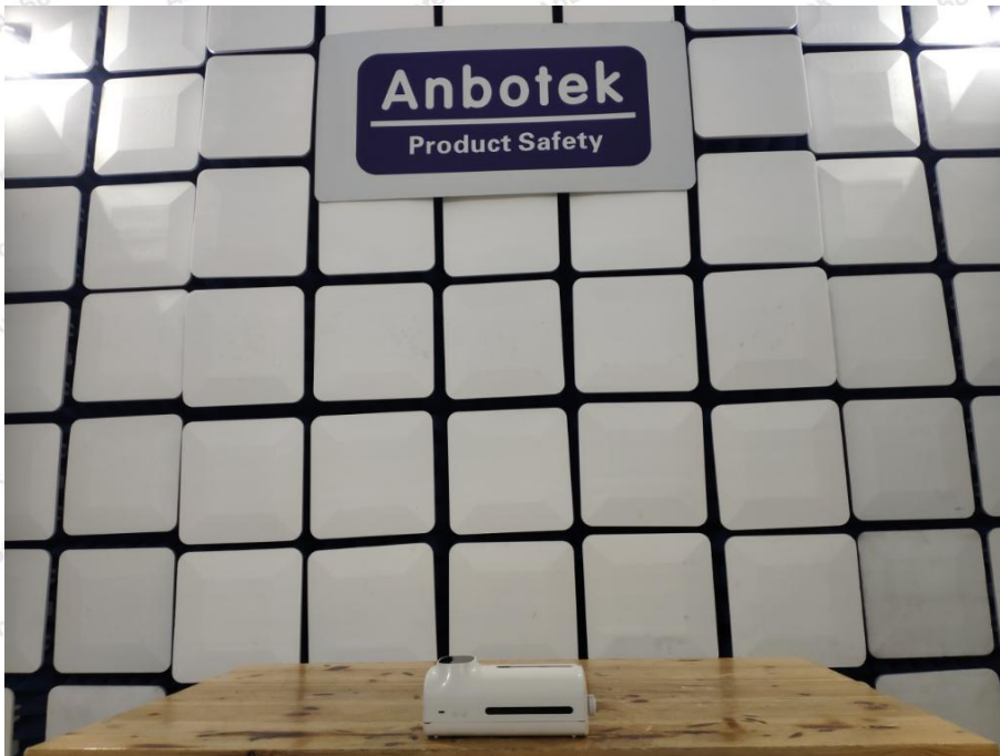
Photo of RF Field Strength susceptibility Test
