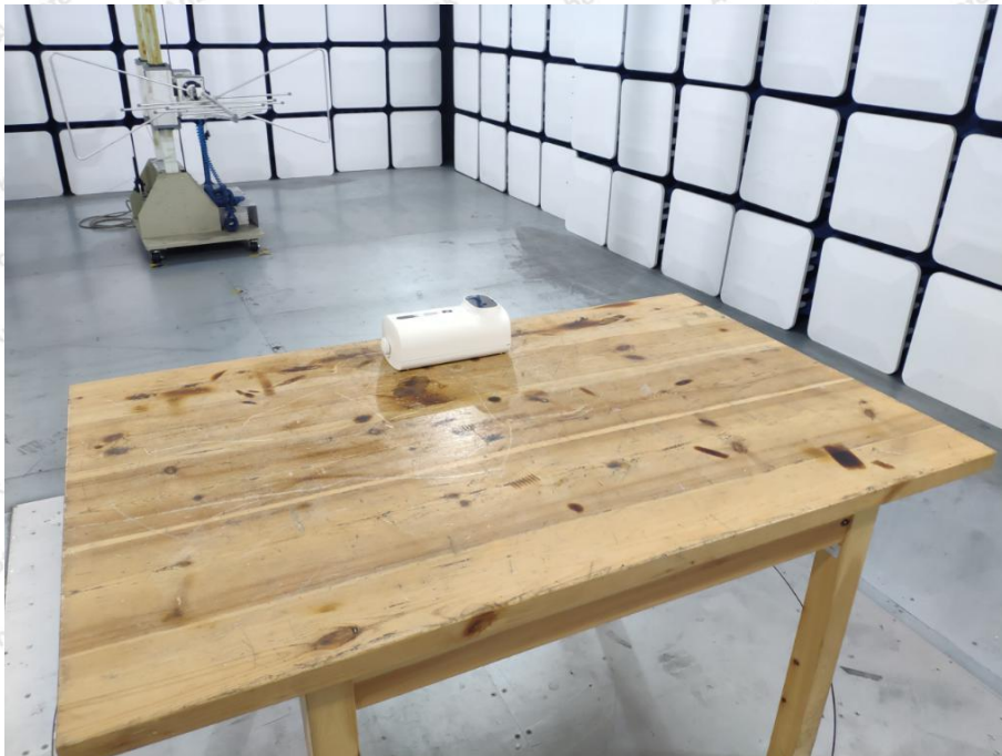
Photo of Radiated Emission Test
