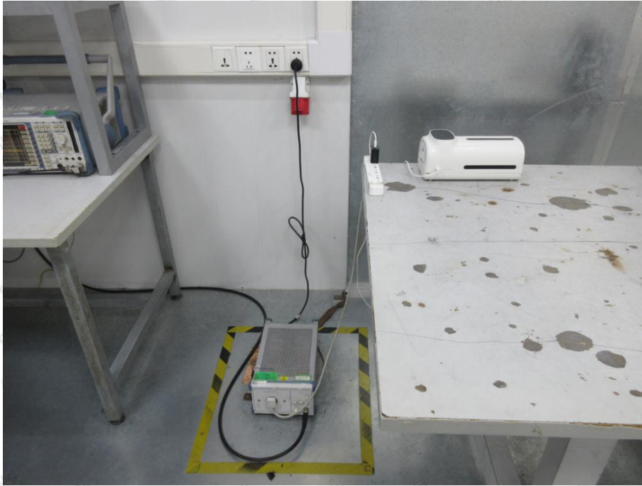
Photo of Power Line Conducted Emission Test
